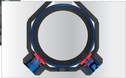
Locking Tabs, Integrated within the Locking Screws, Index Against the Barrel Nut's Channel After Being Tightened, Creating a Rigid 4-Point Steel-on-Steel Lockup
