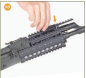
10.Evenly tighten all 4 screws to securely lock the top and bottom covers with the included Allen Wrench.
