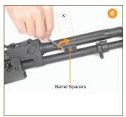
6.Place the 2 Barrel Spacers between the barrel and the gas tube at position X shown in . Tighten the 2 screws to lock the spacers firmly. The Barrel Spacers will prevent over tightening of the top/bottom covers and to allow for normal operation of the piston.
