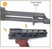
4.Move the Front Holder (Cap) forward and remove the original handguard/ foregrip assembly.
