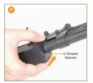
7.Fit as many U Shaped Spacers as needed at the front of the receiver before rails are installed. The spacers should be inserted into the U shaped opening to ensure a tight fit against the barrel.
