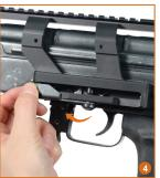
4. Set the Quick Release Lever to the Locked Position (pointing forward) and make sure the mount is completely secured.
