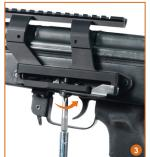
3. The Quick Release Lever at this point should be at the Released Position (pointing rearward) as shown in . Use the screwdriver to gently turn the Adjustment Screw counter-clockwise to achieve a proper tension level. Do not over-tighten.
