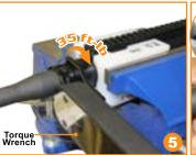
Use the Barrel Nut Wrench to securely tighten the Barrel Nut with enough tension (35 ft-lb). (We recommend using a torque wrench to achieve proper tension).
