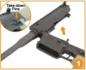
After removal of all necessary parts, use the Take-down Pins on the firearms receiver to Separate the Upper and Lower Receiver.
