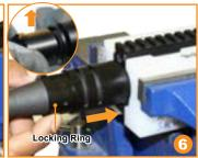
Slide the Locking Ring into the Barrel Nut, making sure the alignment slot on the Locking Ring is vertical and facing upward.
